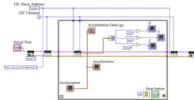
Figure 4. Vibration program using LabVIEW 2019 version student software [17],
