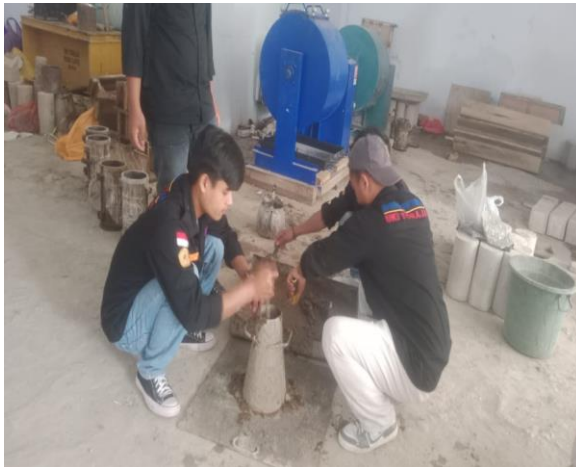
Proses pengujian slump
