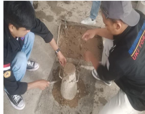
Proses pengujian slump
