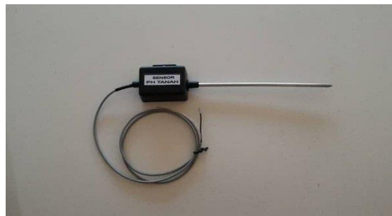
Gambar 2.2 Sensor pH tanah ( https://www.google.com/imgres?imgurl )
