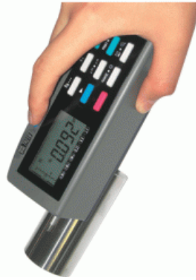
Gambar 2. 13 Surface Roughness Tester Sumber: (Wijayanto, Febriantoko, and Anggono 2016)
