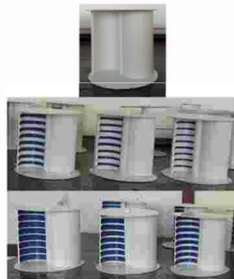
Fig. 2. Eight-grooved blade — 0 mm to 17.5 mm wide
