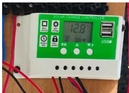
Gambar 3. Solar Charger Controller
