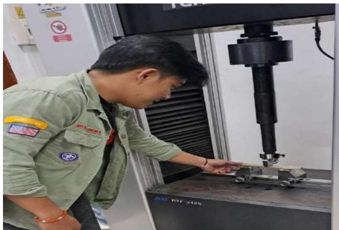
LP 12. Proses pengujian bending
