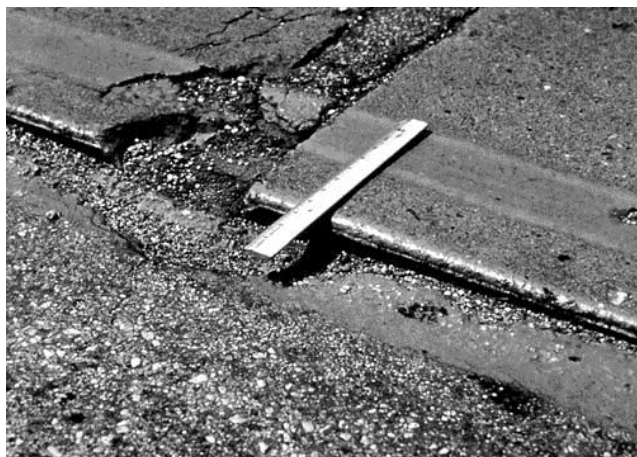
Gambar 2.8. Kerusakan Lane/Shoulder Drop Off
