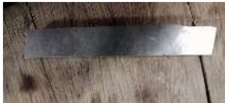
Gambar 2.11 Pahat HSS Bohler Molibdemun Sumber : ( dokumentasi 2025 )
