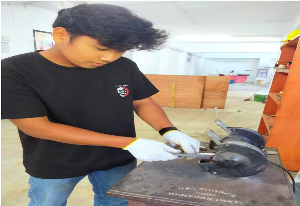
Gambar 3 proses pengasan pahat
