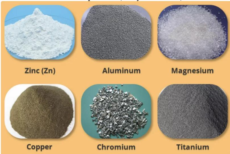
**Gambar 3.2.** Logam Non Ferrous (Hitop Industrial, 2024)
