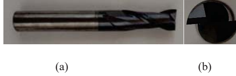
FIGURE 2. (a) endmill two flute (b) the cutting side of the endmill.
