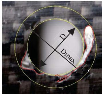
**FIGURE 3.** Delamination on Carbon Fiber Reinforced Polymer (CFRP).
