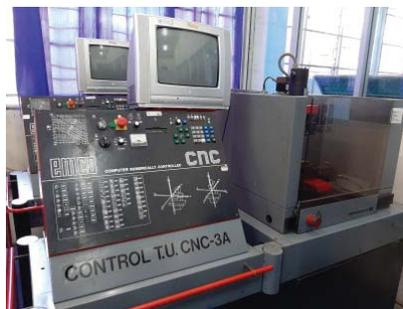
FIGURE 1. Image of T.U. CNC-3A machine.
