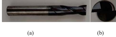
**FIGURE 2.** (a) endmill two flute (b) the cutting side of the endmill.
