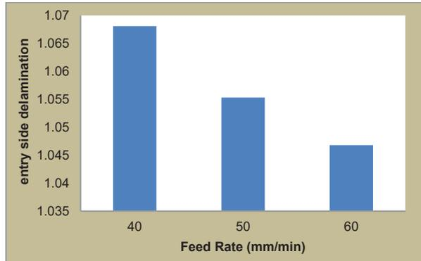
**FIGURE 9.** Graph of entry side delamination factor based on variation of feed rate 40, 50, 60 mm / min (N = 1000 rpm).
