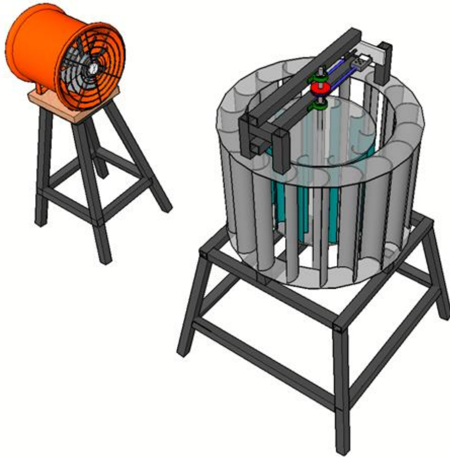
Gambar L. 1 Cylindrical guide vane diameter 500 mm
