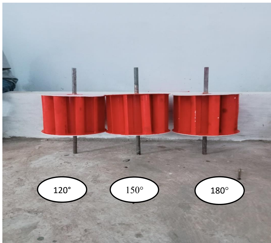
Gambar L.17 Rator kincir air pitchback 10 sudu 120°, 150°, 180°
