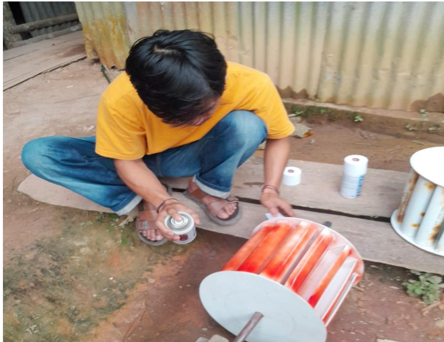
Gambar L.16 Proses pengecatan diameter sudu
