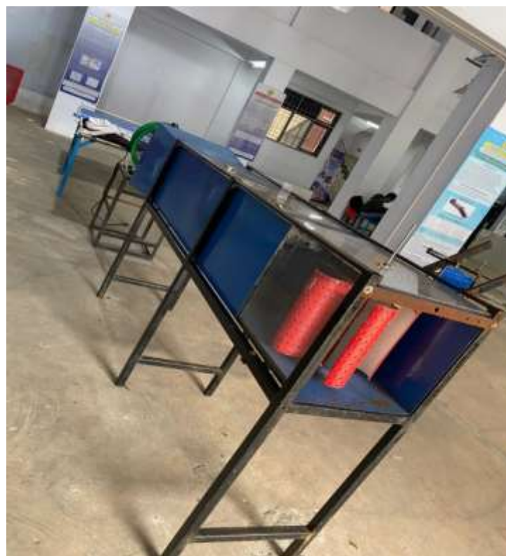
Gambar L.16 wind tunnel turbin angin Savonius tipe L empat sudu variasi diameter dimple tampak samping.
