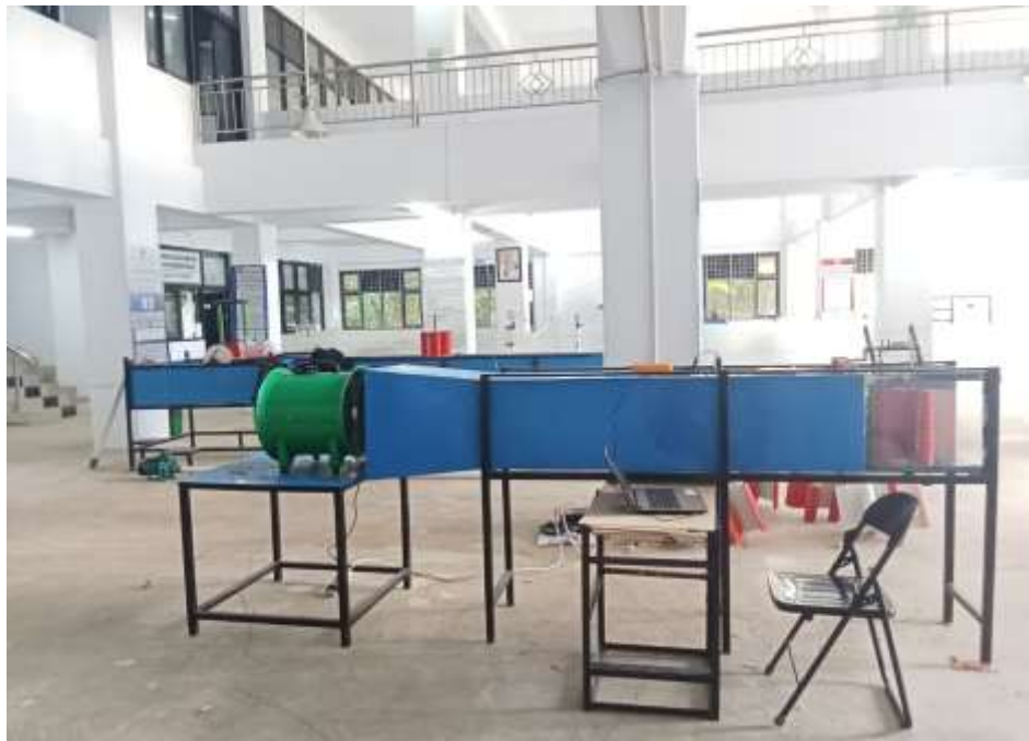
Gambar L.5 Wind tunnel turbin angin Savonius tiga sudu tampak samping
