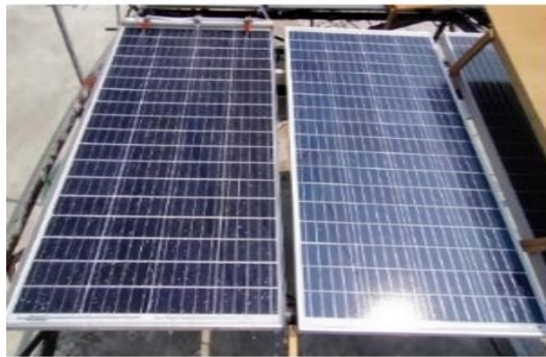
Gambar 2.2 Solar cell jenis polycrystalline Sumber : (Lesmana dkk., 2024)
