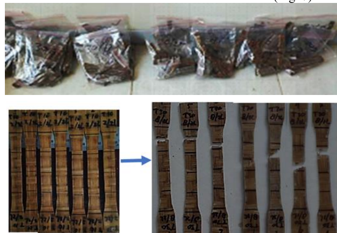
Fig.. 7. Specimen ready for testing
